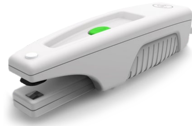
Figure 1 The MultispeQ, a tool to measure plants in their natural environments. Source: photosynq.org
